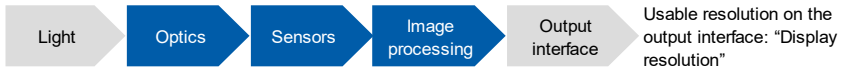
Figure 3-5: The usable resolution on the output interface (resolution of the system) results from the evaluation of the overall path of the flow of information of the light up to the output interface. It is crucial for the proof of capability.
