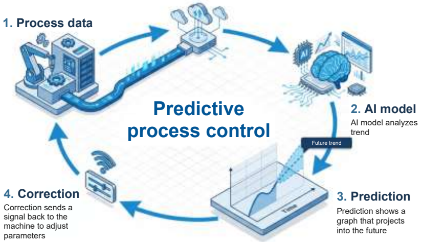
Figure 6-5: AI-powered control loop for predictive process control
