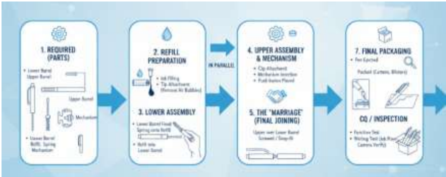
Figure 6-10: Example AI-generated process flow for work instructions – ballpoint pen assembly, derived from spoken employee description
