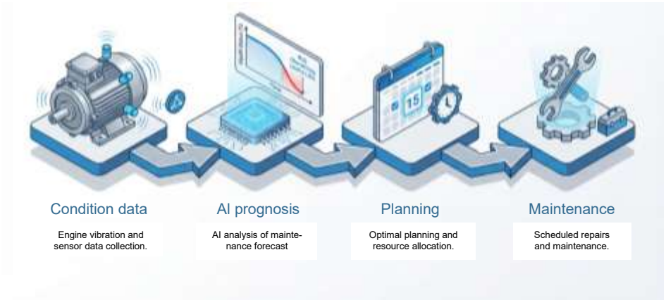
Figure 6-6: Process chain of AI-powered predictive maintenance
