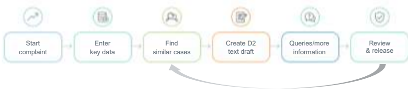
Figure 6-2: Schematic representation of the rule-oriented AI agent workflow in the 8D process
